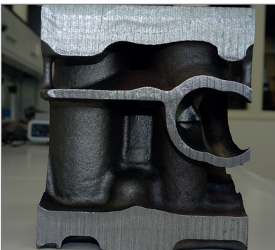
Figure 8. Cast Surface right after shot blasting
